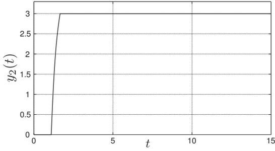
Fig. 5. Time history of  $y_2$  for (16) with the parameters given in Table I. The system is regulated by the controller  $u_2 \in \partial\Psi_S(y_2)$ . The finite-time convergence of  $y_2$  to  $y_d$  is verified.
