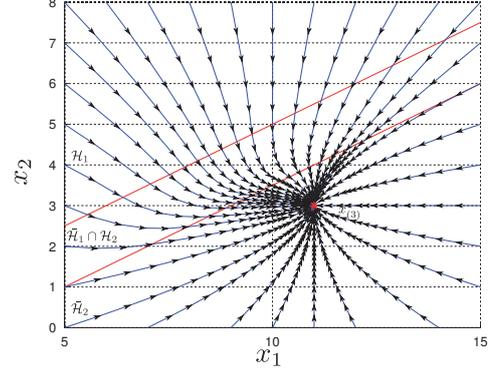
Fig. 4. Phase plane of (16) with the parameters given in Table I. Regulation is achieved with the controller  $u_2 \in \partial\Psi_S(y_2)$ .
