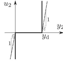
Fig. 2. Graph of the multifunction  $U(y_2) = \partial\Psi_S(y_2)$  (solid line) and a continuous approximation (dotted).
