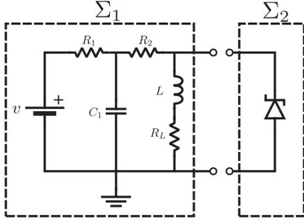
Fig. 3. An RLC circuit with a source. The goal is to regulate the voltage at the port of  $\Sigma_1$ .
