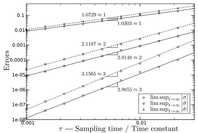
Fig. 6. Third-order sliding mode. Order of the errors as functions of the sampling period (solid) and the actuator time-constant (dashed). The error order for  $\sigma$  matches well with the sliding-mode order.
