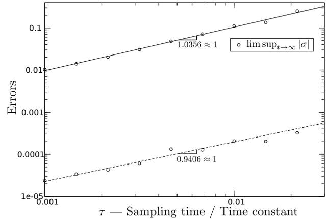
Fig. 2. First-order sliding mode. Order of the error as a function of the sampling period (solid) and the actuator time-constant (dashed). The error order matches the sliding-mode order almost exactly.
