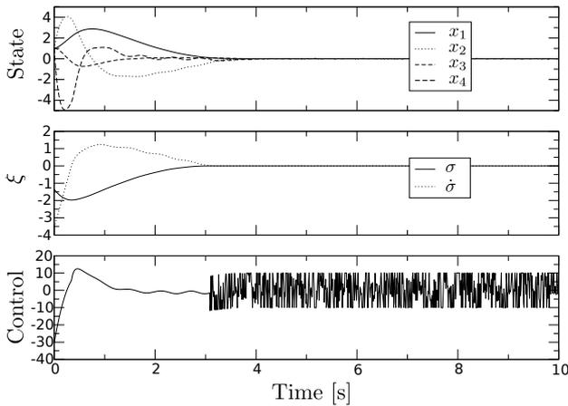
Fig. 3. Simulation results for a second-order sliding mode controller. The system is perturbed by  $w = 0.5 \sin(10t)$ . The control (10) is sampled and held every  $\tau = 0.001$  seconds.
