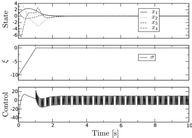
Fig. 1. Simulation results for a first-order sliding mode controller. The system is perturbed by  $w = 0.5 \sin(10t)$ . The control (4) is sampled and held every  $\tau = 0.001$  seconds.
