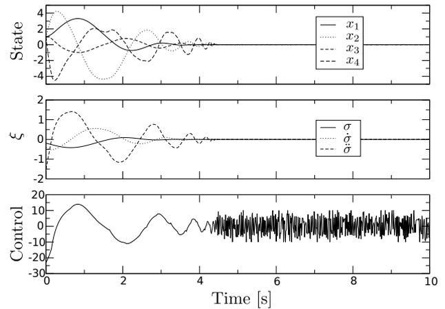
Fig. 5. Simulation results for a third-order sliding mode controller. The system is perturbed by  $w = 0.5 \sin(10t)$ . The control (11) is sampled and held every  $\tau = 0.001$  seconds.
