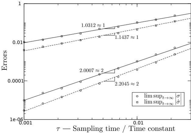
Fig. 4. Second-order sliding mode. Order of the errors as functions of the sampling period (solid) and the actuator time-constant (dashed). The error order for  $\sigma$  matches well with the sliding-mode order.
