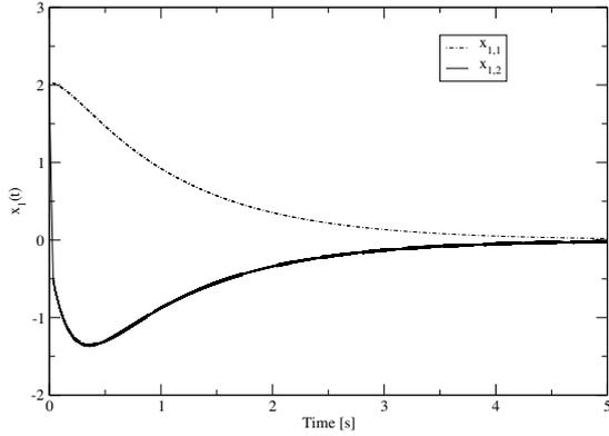
Fig. 2. Response of the nominal system  $\dot{x}_1 = A_1 x_1 + B_1 u_1$ .
