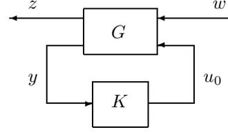
Fig. 1. General Block Diagram of a Control System.
