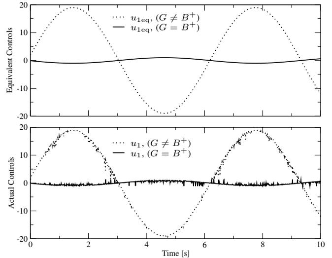
Fig. 2. High frequency controls. Equivalent controls (upper) for  $G \neq B^+$  (dotted) and  $G = B^+$  (solid). Actual controls (lower)  $u_1 = -35s/(|s| + 0.0002)$  for  $G \neq B^+$  (dotted) and  $u_1 = -1.5s/(|s| + 0.0002)$  for  $G = B^+$  (solid).
