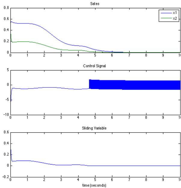
Fig. 4. Simulation results with  $k_1 = 10$ ,  $k_2 = 1.5$  and small initial conditions
