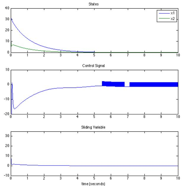
Fig. 2. Simulation results with  $k_1 = 60$  and  $k_2 = 1.5$
