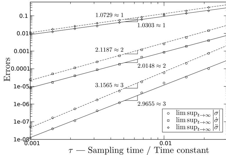
FIGURE 6. Third-order sliding mode. Order of the errors as functions of the sampling period (solid) and the actuator time-constant (dashed). The error order for  $\sigma$  matches well with the sliding-mode order.
