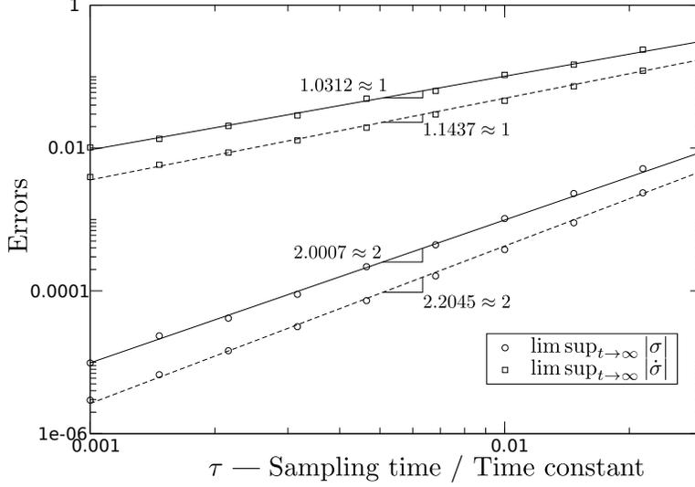
FIGURE 4. Second-order sliding mode. Order of the errors as functions of the sampling period (solid) and the actuator time-constant (dashed). The error order for  $\sigma$  matches well with the sliding-mode order.
