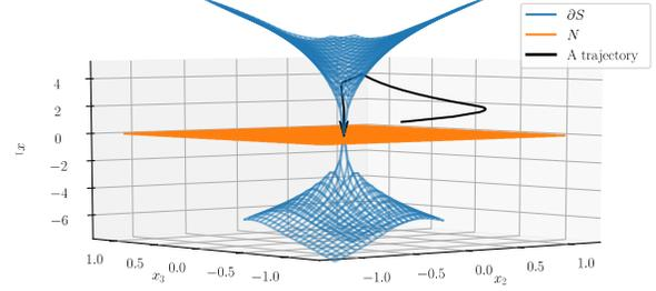
Fig. 1. Hyperplane  $N = X_1^+ \cap X_1^-$  (solid orange) and boundary of the forward invariant and finite-time attractive set  $S$  (blue wireframe). A trajectory is also depicted (solid black arrow). The initial state lies outside of  $S$ , so the controller drives  $x$  away from  $N$  until it reaches  $S$ . The controller then keeps  $x$  in  $S$  and steers it towards the origin in finite time.
