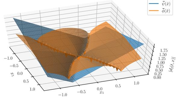
Fig. 2. Linear and nonlinear sector boundaries arising from  $\bar{\psi}$  and  $\bar{\phi}$ , respectively.
