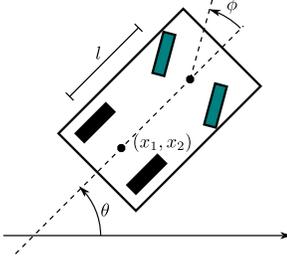
Fig. 3. Kinematic model of a car. The car configuration is parameterised by the Cartesian coordinates of the centre of the rear axle, the angle of the main body with respect to the horizontal, and the steering angle with respect to the main body. The control inputs are the linear velocity and the steering angular velocity.
